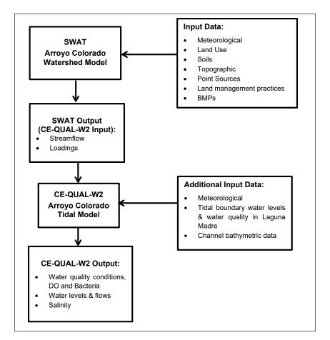
Figure 9.1. Schematic of modeling system
